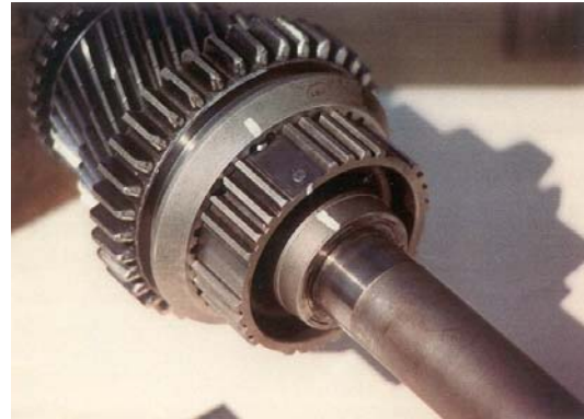
Second synchro sleeve with stop pin rivet added between paint marks. This was added to all gearboxes from Dec 1952 to prevent overtravel when shifting into first; reference Service Bulletin No. 116
